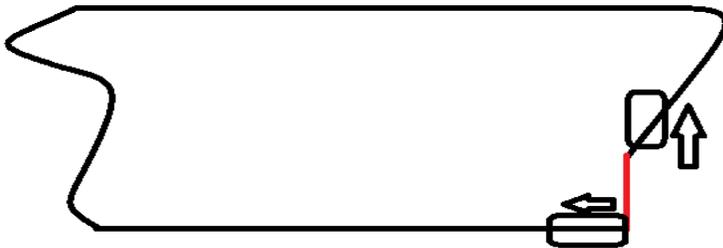
Once the robot reaches the color it will not take that path. Since we attached sensors the back portion of the robot we will use those sensors to follow the path instead and go the other way. The sensors will allow the robot to detect the line and continue following it with the motors. The caster wheel will assist the robot if there is any need to make any turns in the path. If there isn't a caster wheel then the robot will not be able to make sharp turns or turn at all.
