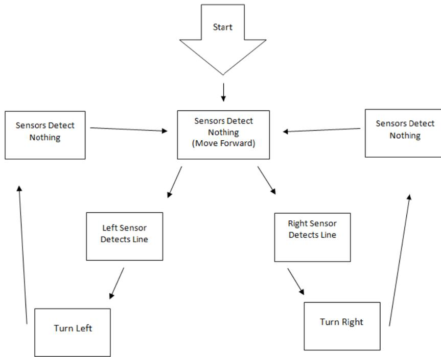
**Comment [L3]:** This diagram is good. It clearly shows the action flow when the robot functions.
