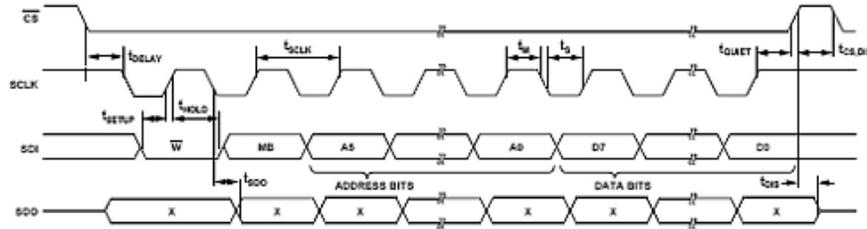
Figure 5. SPI-4-Wire Write
