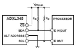
Figure 8. I<sup>2</sup>C Connection Diagram (Address 0x3B)
